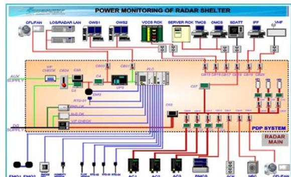
Figure 6 : Power Flow Monitoring Window
