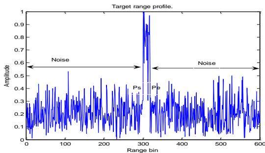
Figure 1 High range resolution profile of an air target.
