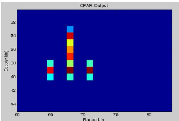
Figure 7: CFAR Output without Gaussian Centroiding
