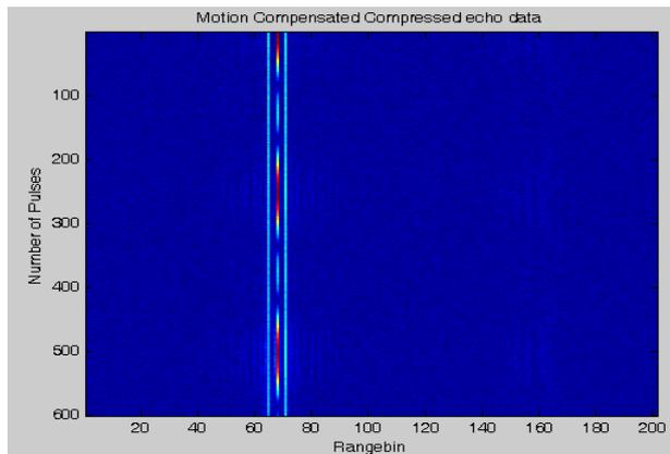
Figure 6: Output of Motion Compensated Compressed data
