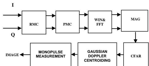
Figure 3: Block diagram of RAID Assesment SP Algorithm
