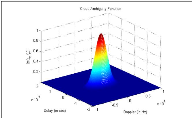
Figure 5 3D Ambiguity Function for Matched Filter
