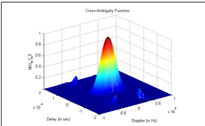
Figure 6 3D Spread Ambiguity Function for Colored Noise Matched Filter for  $X(f)$
