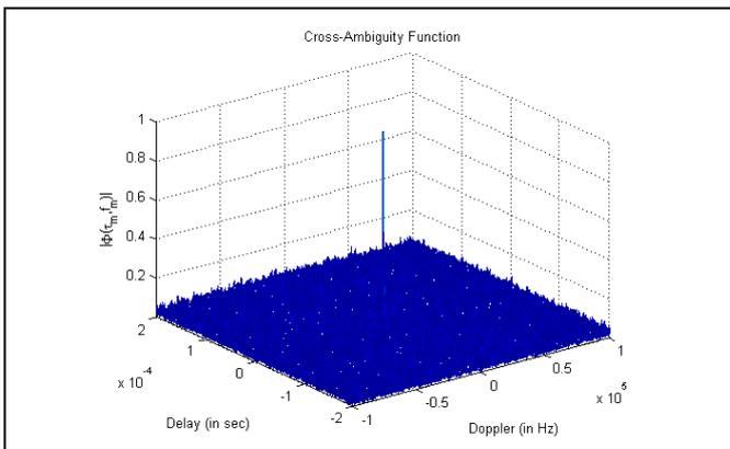
Figure 7 Spread Ambiguity Function for Colored Noise Matched Filter for SINR-MI waveform
