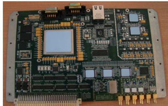
Figure 3: waveform generator card
