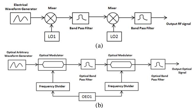
Figure 1: Exciter chain in radar (a) conventional using electrical component <sup>[1]</sup> (b) using optical interface
