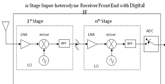
Fig: 1. Super-heterodyne receiver front end.
