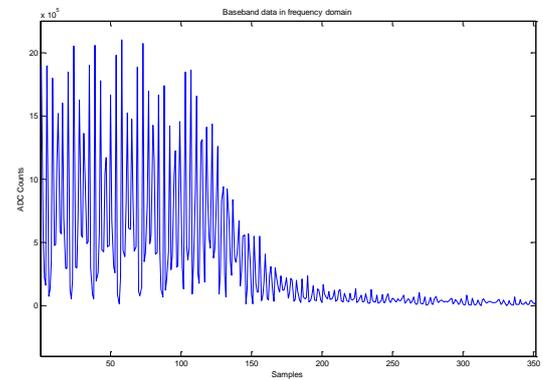
Fig: 8. Signal after down conversion in frequency domain.
