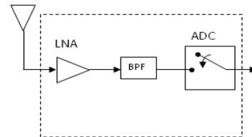
Fig: 2. Direct RF sampling receiver front end.
