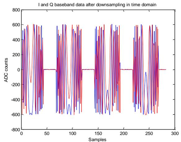
Fig: 9. I and Q baseband data after down sampling in time domain.
