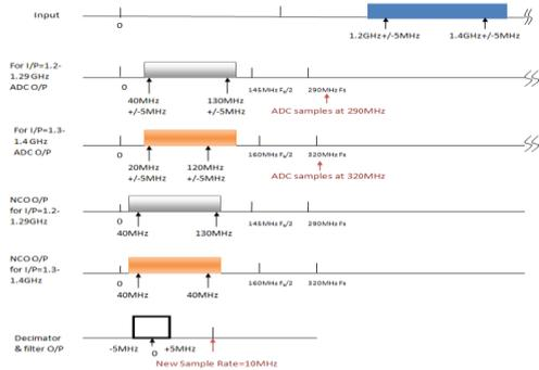
Fig: 4. Direct RF sampling with single sampling frequency.
