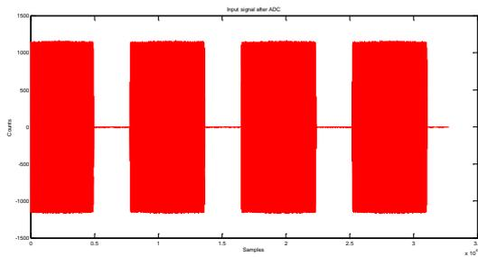
Fig: 5. RF signal after sampling using ADC in time domain.
