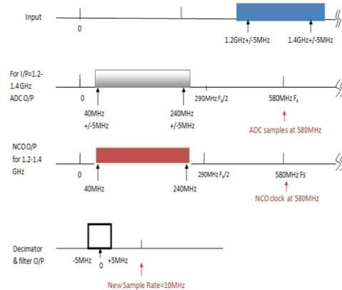
Fig: 3. Direct RF sampling with single sampling frequency.
