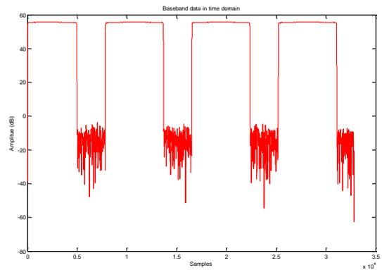
Fig: 7. Signal after down conversion in time domain.
