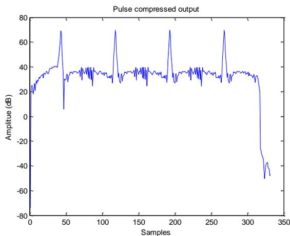
Fig: 11. Pulse compressed output for 10us LFM pulse.
