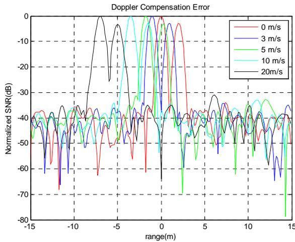
Fig. 4. Doppler Compensation error effect
