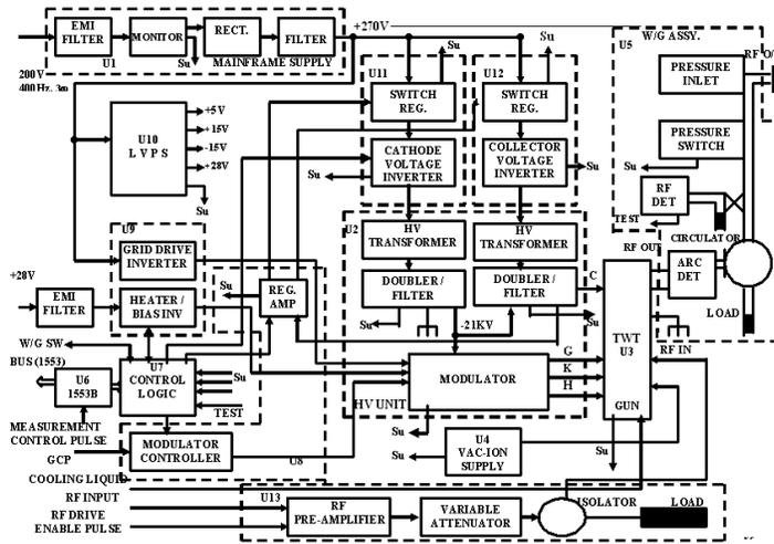
Fig.1 Transmitter Block diagram
