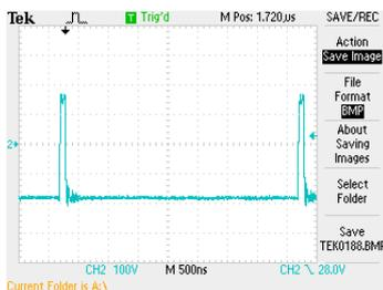
Figure 7. Grid voltage swing at 250KHz PRF
