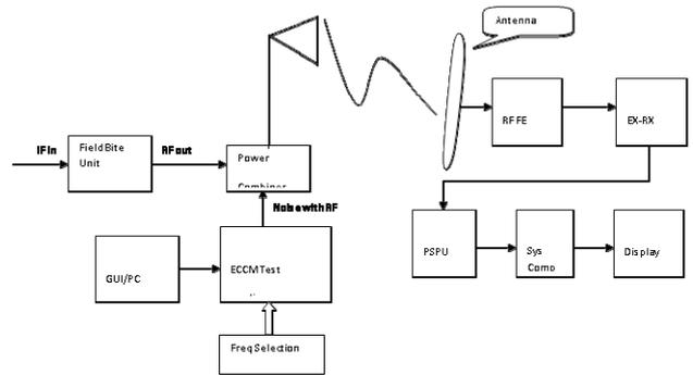
Fig 2: ECCM test jig introduced
