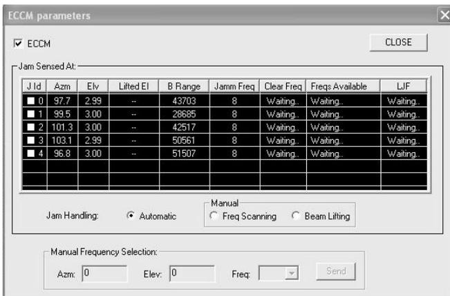
Fig 5: Display showing Jammed Frequencies
