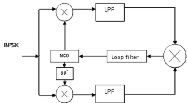
Fig. 3 Costas loop for BPSK Demodulation
