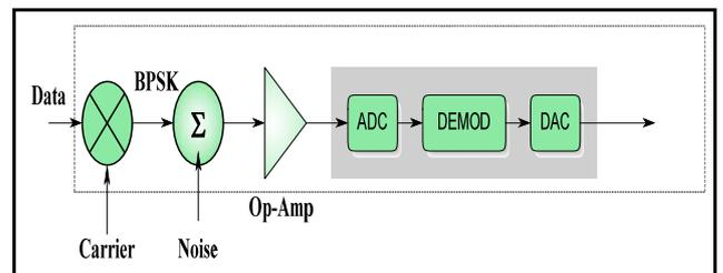
Fig. 10 Set-up for verifying Band-Pass Sampling
