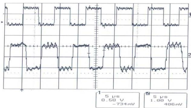
Fig. 13 Modulating and Demodulated Signal for Square data with LPS
