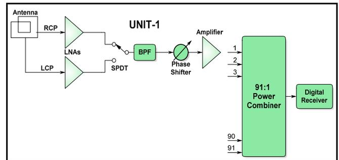
Fig. 1 RF Front end of MEOLUT: Conventional Approach
