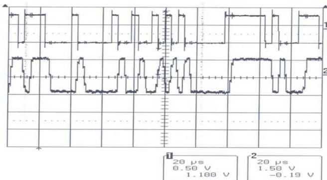
Fig.11 Modulating and demodulated signal for PRBS data with BPS
