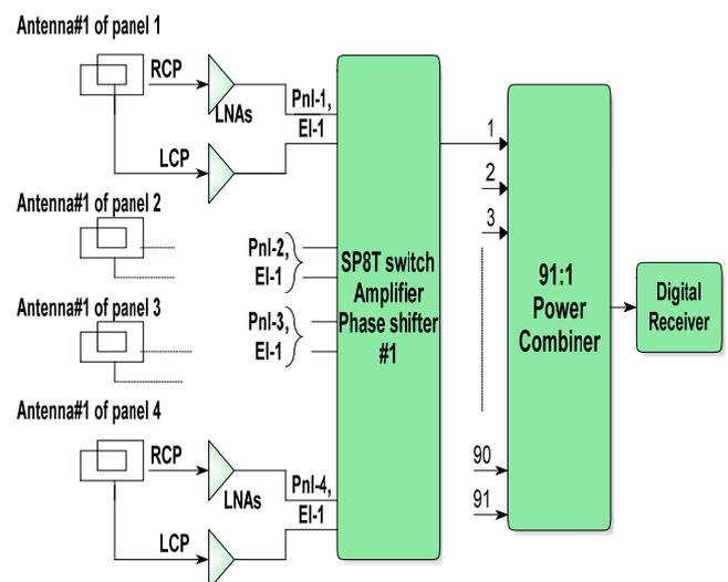
Fig. 2 RF Front end of MEOLUT: Hardware Sharing Approach
