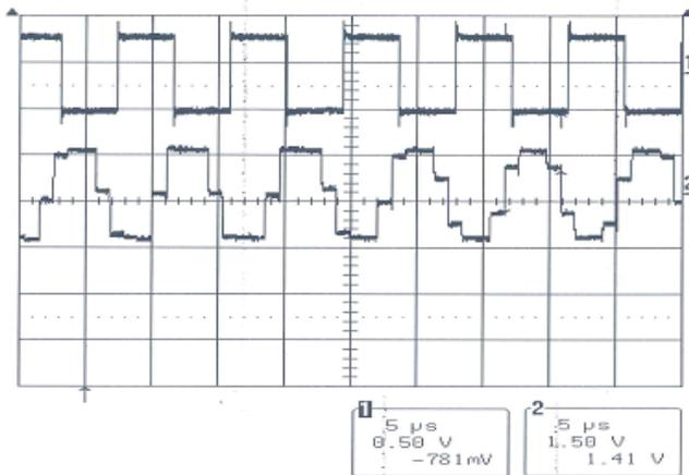
Fig. 12 Modulating and Demodulated Signal for Square data with BPS
