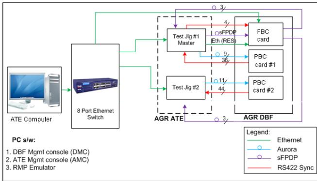
Figure 1. DBF Test Setup
