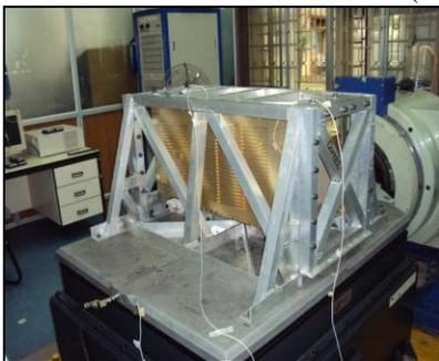
Figure 2. DBF Vibration Test Setup
