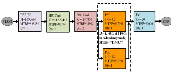
Figure 4. Reliability Block Diagram-DBF
